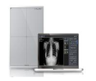
This device allows for X-rays to be done without having to move the newborn, who might have multiple catheters or drains, which can be difficult to immobilize. The detector is simply placed inside the cassette at the bottom of the incubator.
