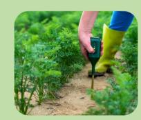
Using a tensiometer to determine how much water is stored in the soil
