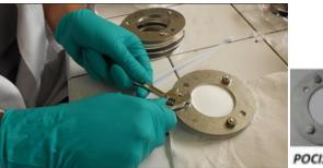
The POCIS was built using Oasis® HLB bulk sorbent (average particle diameter: 60 µm) and polyethersulfone (PES) SUPOR 100 membranes (0.1 µm, 90 mm diameter) PRC: DIA-d5
